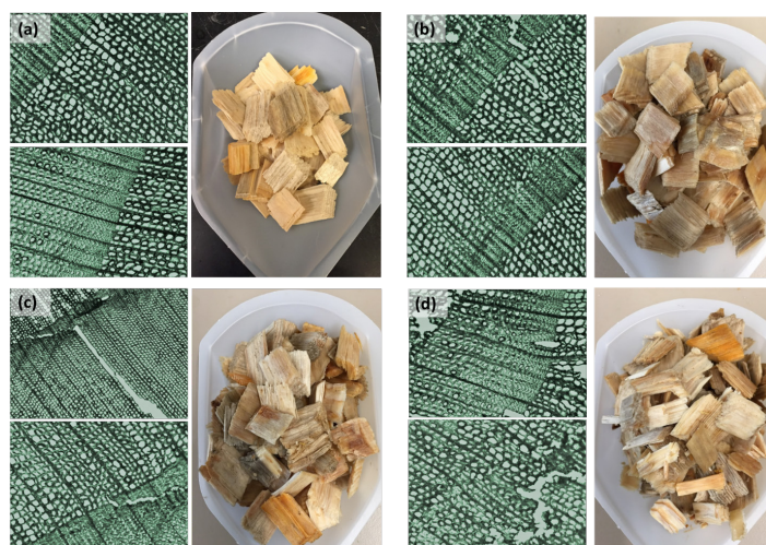
Figure 5: Microscopy samples from (a) Control chips. (b) Wood chips compressed at 3:1 compression ratio. (c) Wood chips compressed at 5:1 compression ratio, and (d) Wood chips compressed at highest compression ratio of 6:1.
